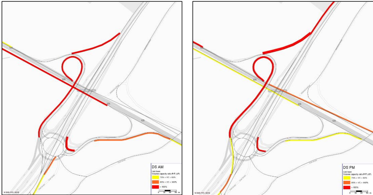
Figure 3-24: M2J5 2041 Do Something Link V/C Performance (AM Peak left, PM Peak right)
