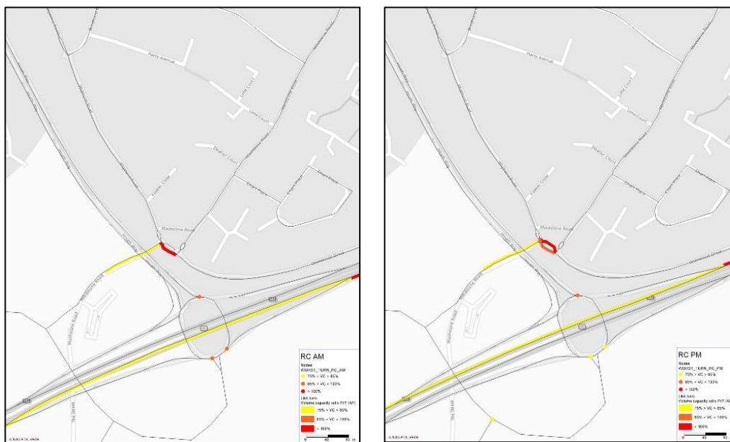
Figure 3-17: M2J4 2041 Reference Case Link V/C Performance (AM Peak left, PM Peak right)
