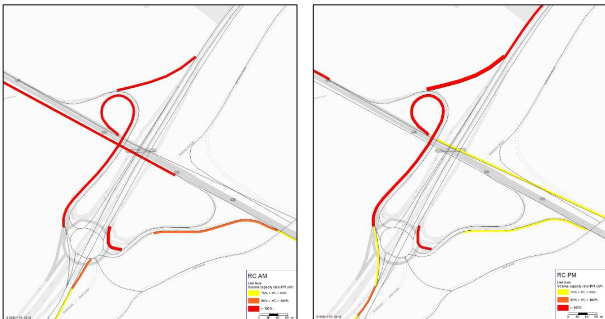
Figure 3-23: M2J5 2041 Reference Case Link V/C Performance (AM Peak left, PM Peak right)
