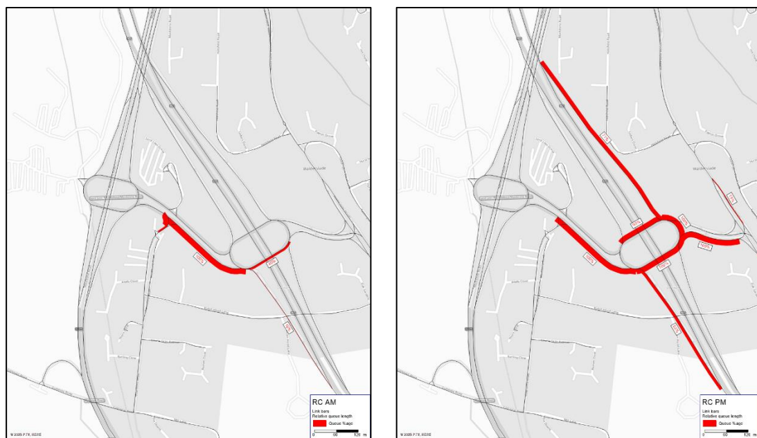
Figure 3-12: M2J3 2041 Reference Case Link Relative Queues (AM Peak left, PM Peak right)
